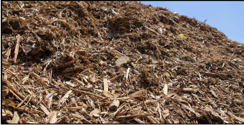
Figure 7: Unsaleable mill residues can look like this but vary in composition, sizes, and moisture content. A large proportion of this residue is in the form of sawdust. Historically, mill waste that could not be sold as byproducts was burned in “tipi burners.” During the height of timber harvest in Humboldt County, approximately 200 mills were operating – and each had a “tipi burner” that burned mill residues around the clock. During this era, a great deal of unfiltered smoke was emitted. Many of these burners can still be seen today at old mill sites.
