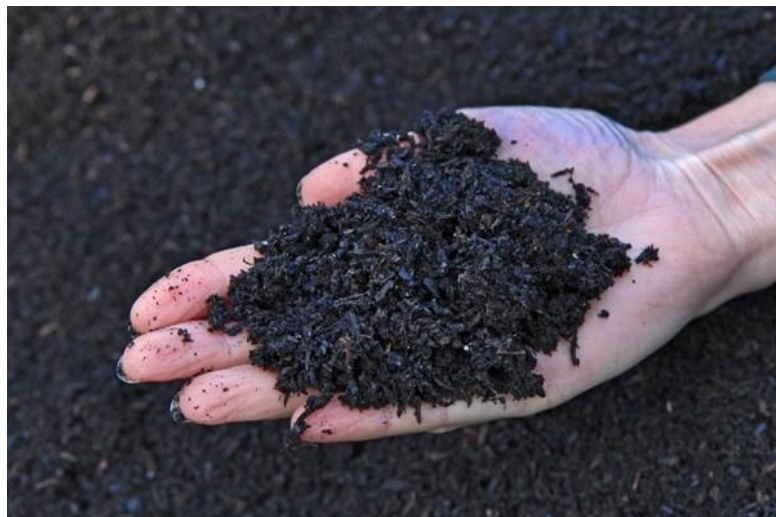
Figure 11. Biochar is black, highly porous, lightweight, fine-grained and has a vast surface area. Approximately 70% of its composition is carbon. The remaining material consists of nitrogen, oxygen, hydrogen and other elements. Biochar's chemical composition varies depending on the feedstocks used to make it and methods used in pyrolysis.
