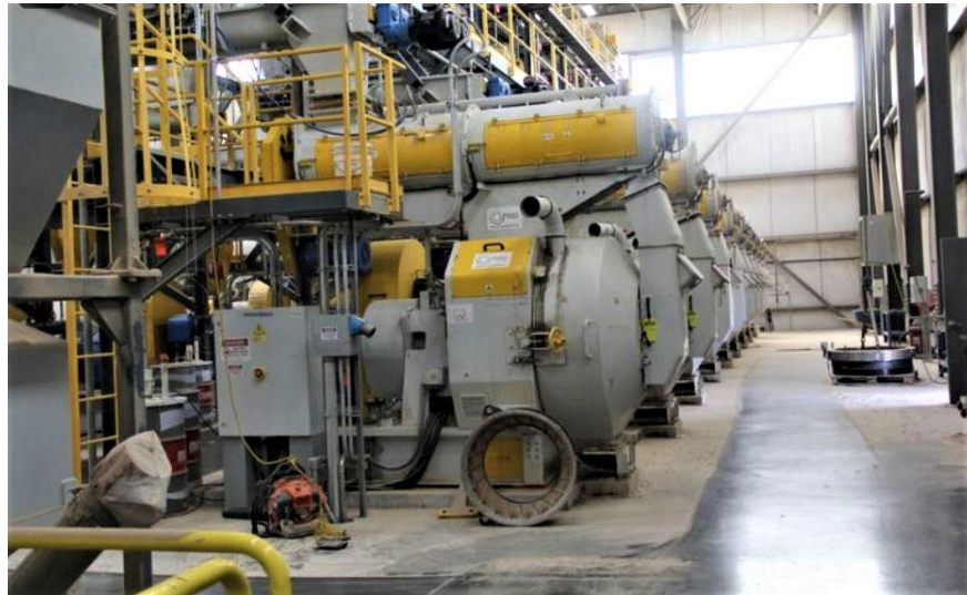
Fig. 20. A pellet manufacturing facility which utilizes multiple pellet mills in a parallel system ( Index Journal 2020 )
