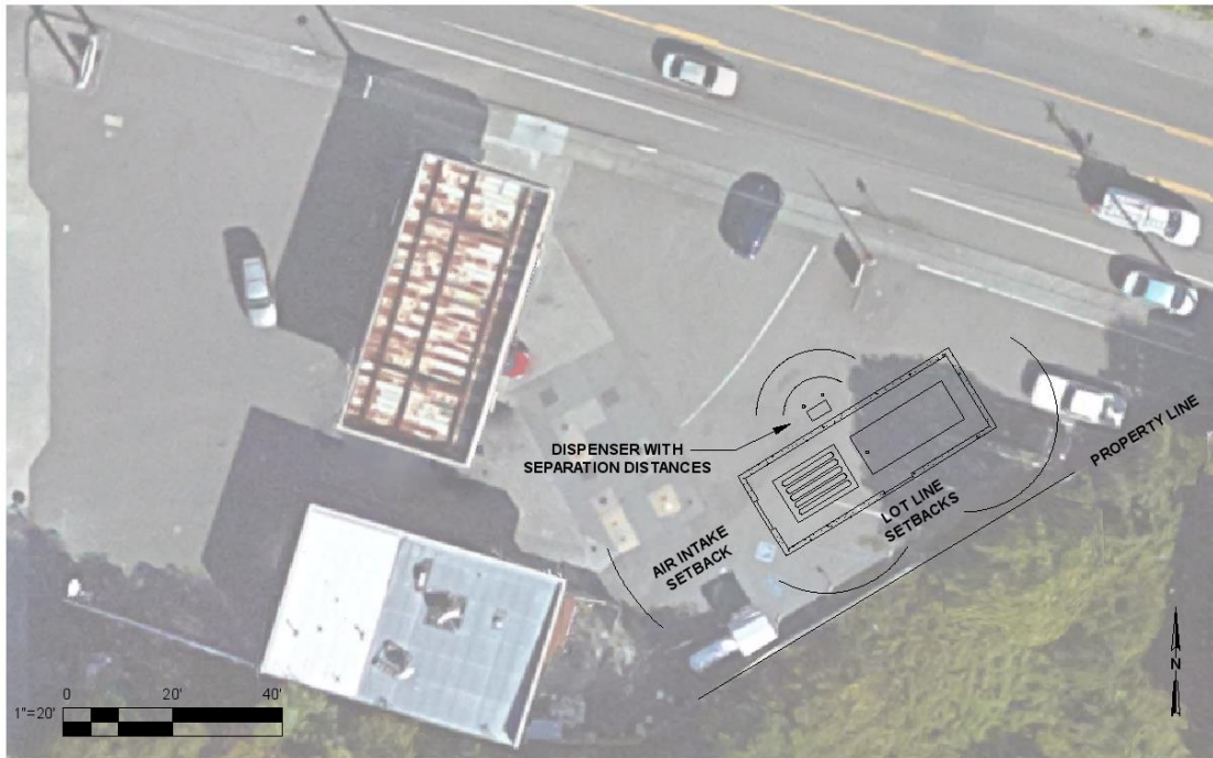
Figure 16: Dimensionalized Layout of a Gas-delivered Station at Myrtle Shell
