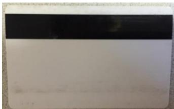
**Step 8:** Insert the test card that came with the Payment Module into the Payment Module card reader to put the module into test mode.
