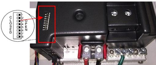
**Step 7:** Slide the EVSE's GFI Dip Switch number 3 to **Open** to put it into ZigBee Setup Mode. After a few moments, all the lights on the Control Module will begin flashing, letting you know the EVSE is now in ZigBee Setup Mode.
