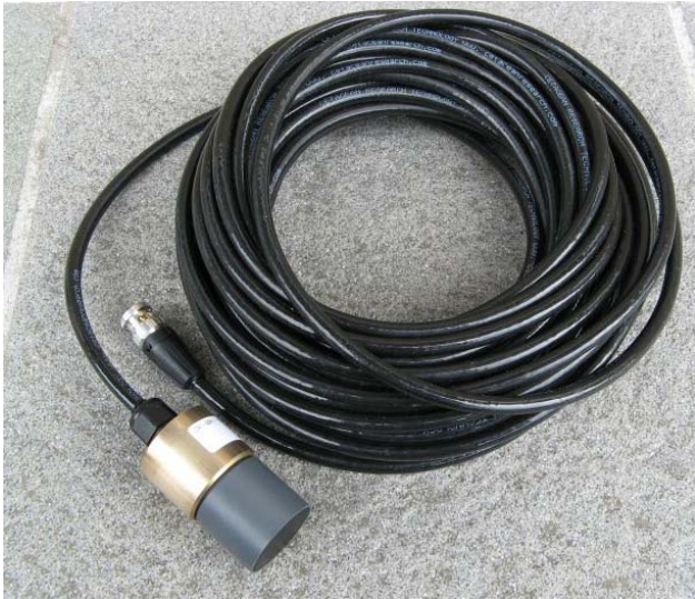
Typical hydrophone and cable for boat deployment.
