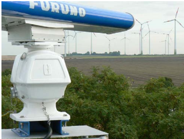
Marine-type radar at a wind farm in Germany (Borst 2008)
